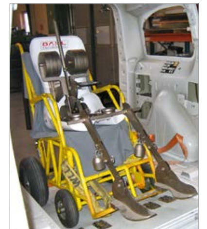
ECE regulation 17 H-point measurement
